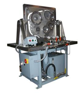
Prior to building this system IFS worked with the gearbox manufacturer to establish the flow rate, temperature requirements and oil quality required to meet Rolls-Royce specifications. Test tooling was included as part of the package.
